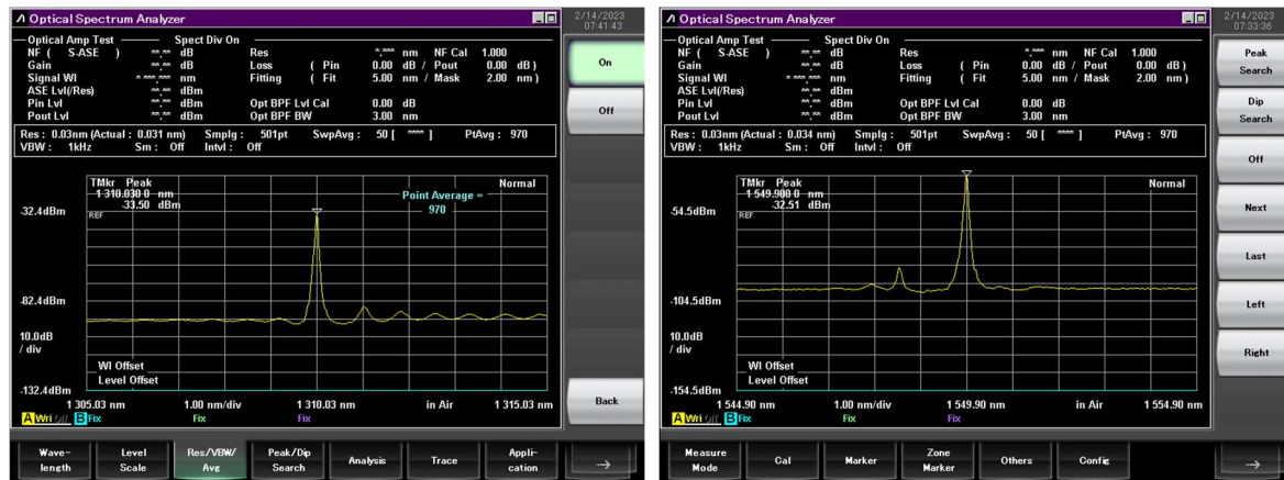
Figures 3. Measurement results of the laser sources with a wavelength of 1310 nm (left side) and 1550 nm (right side).
